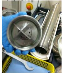
d. Place rotor carefully on the spindle. Be very careful not to knock the top of the centrifuge, and use dark gray screw cap to protect the metal bearings.
