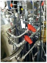
10) While this happens, sterilize all ports ONE AT A TIME for 10-20 seconds. First, open red valve associated with the port, wait five seconds, then open blue valve. After 10-20 seconds minimally (or until the valve is hot to the touch – BE CAREFUL if you touch the valve! Jie recommends 1 min) close the red valve, wait five seconds, and close blue valve.
