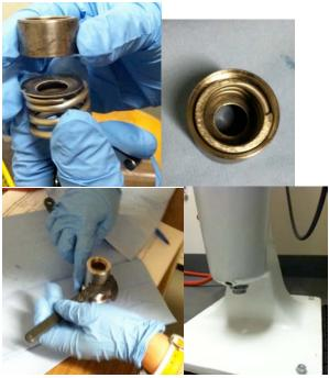
c. Then assemble the centrifuge tube. Follow the picture in the manual to place the teflon sheet in correctly. This is very important because there will be cell loss if improperly placed.
