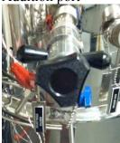
b. Sampling port (does not have blue valve associated with it.)
